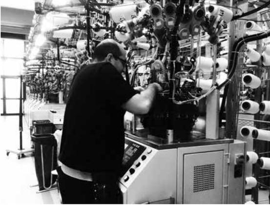
A knitting expert checking the workings of a circular-knit knitting machine.
